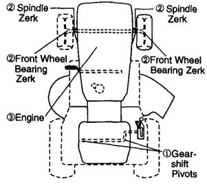
**®SAE 30 or 10w30 MOTOR OIL** *QGENERAL PURPOSE GREASE* **③REFER TO Maintenance "ENGINE" SECTION IMPORTANT:** Do not oil or grease the pivot points which have special nylon bearings. Viscous lubricants will attract dust and dirt that will shorten the life of the self-lubricating bearings. If you feel they must be lubricated, use only a dry, powdered graphite type lubricant sparingly.
